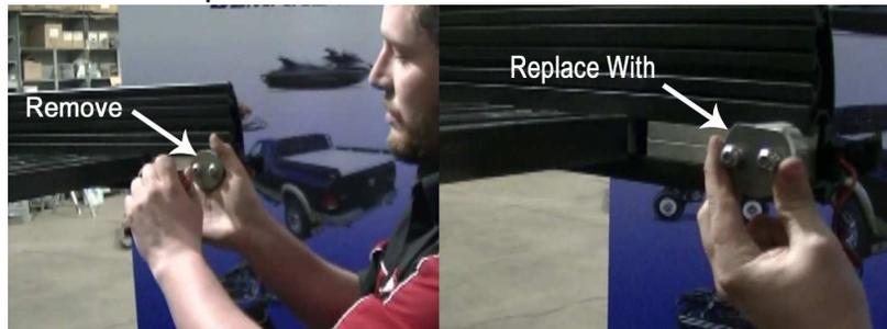
2.4 **Add hardware onto the TRUCKBOSS deck.** -- On each side, four 5/16 by 3/4" bolts will be added to the surface of the deck and two knobs with 1" carriage bolts will be added to the deck sides. The two 3/4" carriage bolts should be added into each of the two rear capture channels on each side. The knobs should be added into the lower of the two capture channels on the each of the sides.
