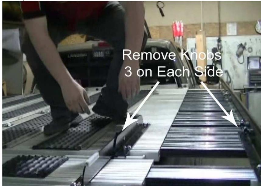
2.14.3 This allows the side arm to be moved inwards. Repeat the process on the other side.
