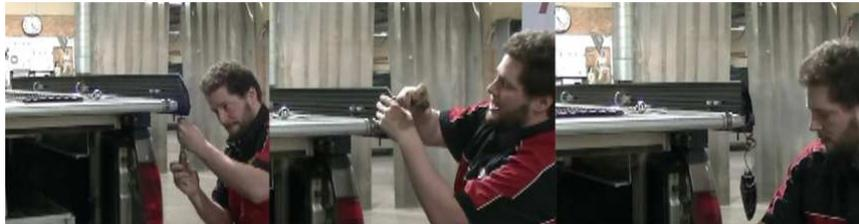
1.2 Using a 1/2" socket, remove any D-Rings located in the rear two modules of the TRUCKBOSS deck surface and/or in the back half of the TRUCKBOSS sides.
