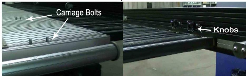
2.5 Lift the main extension out of the box. Remove the wood shipping blocks off of both sides
