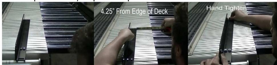
**2.8 Install the pull-out sides in to the main extension assembly.** Slide the sides into each side of the main assembly.
