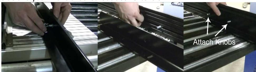
2.13 With the deck extension now locked in the out position the sides can be shut. The angle bracket on the extension will prevent the side from going all the way in. This is normal and the way that it was designed.
