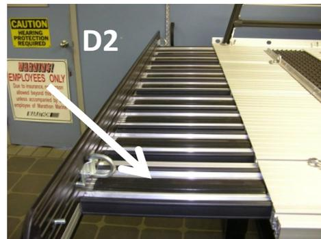
**D-3** Insert 8 plastic T-Nuts into each of the rearmost 5 capture channels on your deck surface (TRUCKBOSS 8) or 8 plastic T-Nuts into each of the rearmost 4 capture channels on your deck surface (TRUCKBOSS 7).
