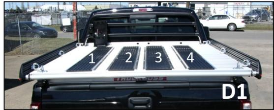
Note: The four strips are aligned on the deck so that a single sled load will use #1, and #4. When two sleds are loaded the left sled will use #2 and the extended side and the right sled will use #3 and the extended side. The measurements used in these instructions will accommodate most snowmobiles. Adjustments in placement may be necessary for some models of snowmobiles.
