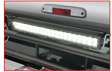
Capture channels are used to add popular add-on such as carbide kits, deck hooks, and lights.
